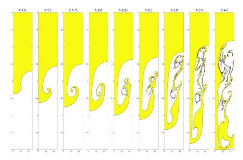
FIGURE 1. A low Atwood ratio problem of Algorithm 1 with finite element  $(\mathcal{P}^1, \mathcal{P}^1, \mathcal{P}^1)$  for  $(\mathbf{u}, p, \rho)$  at Re = 1000 (density contours  $1.4 \le \rho \le 1.6$ )
