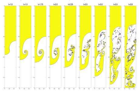
FIGURE 2. A low Atwood ratio problem of Algorithm 1 with finite element  $(\mathcal{P}^1, \mathcal{P}^1, \mathcal{P}^1)$  for  $(\mathbf{u}, p, \rho)$  at Re = 5000 (density contours  $1.4 \le \rho \le 1.6$ )
