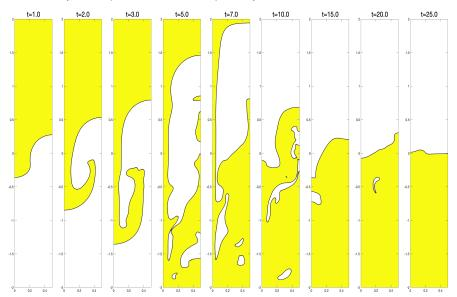
FIGURE 4. A low Atwood ratio problem of Algorithm 4 with finite element  $(\mathcal{P}^1, \mathcal{P}^1, \mathcal{P}^1)$  for  $(\mathbf{u}, p, \rho)$  at Re = 1000 (density contours  $1.4 \le \rho \le 1.6$ )
