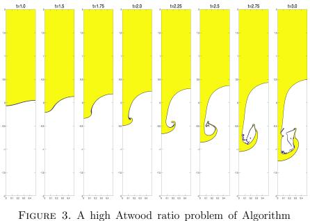
FIGURE 3. A high Atwood ratio problem of Algorithm 1 with finite element  $(\mathcal{P}^1, \mathcal{P}^1, \mathcal{P}^1)$  for  $(\mathbf{u}, p, \rho)$  at Re = 1000 (density contours  $2 \le \rho \le 4$ )
